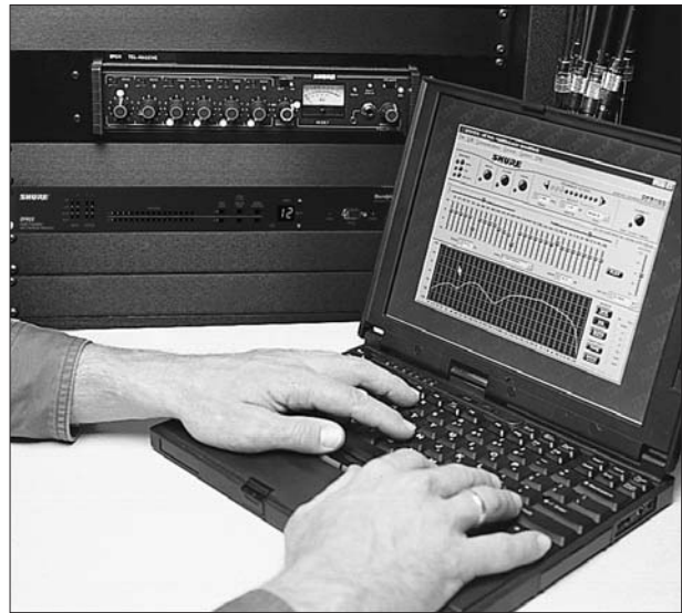
Example of a PC-controlled Feedback Reducer and Equalizer. (Shure DFR22 shown on bottom of rack.)
